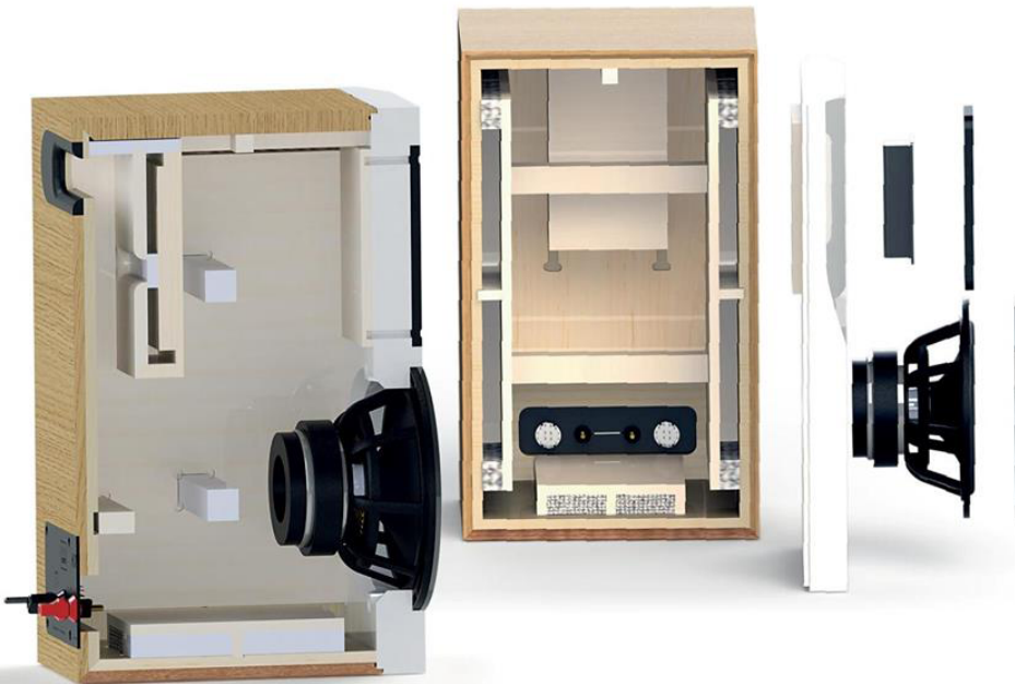
ABOVE: Renderings from the side, front and exploded baffle reveal the lightly braced Helmholtz cavities employed to both control resonances and modify the port output at the cabinet rear
