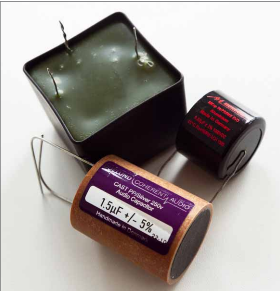
A few of the gems used on the crossover of the „Episode 2“. The potted transformer at the top is still a prototype
